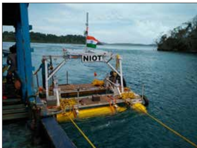
Figure 4: Current Turbine Testing in Andaman
